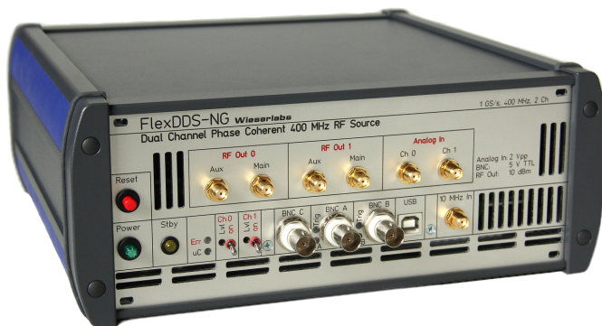
Figure 1.1: The FlexDDS-NG DUAL (left) and the dual-channel AD9910 RF generator slots (right) of the FlexDDS-NG Rack are functionally equivalent.
